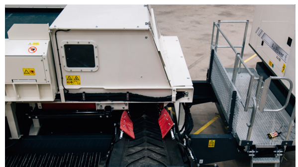
Movable splitter box allowing optimal material flow whilst enabling the machine to fold within 3m wide transport width
