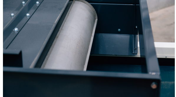
Variable speed 2m (6' 7") wide high strength neodymium radial pole drum for optimal ferrous metal recovery
